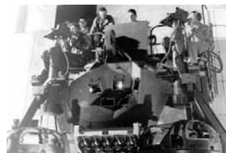
▲ Fred Waller's artillery simulator (above) used five 35mm projectors to create "targets" — aircraft. A roller-coaster ride: the Cinerama screen (top) allowed the audience to get close up to the action
